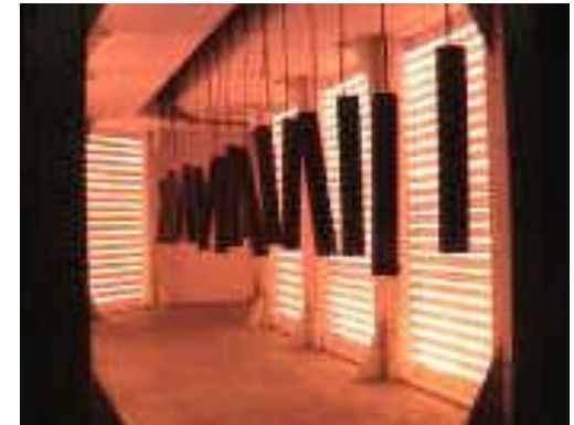
Electric IR Tunnel Oven for Powder Coat Curing
